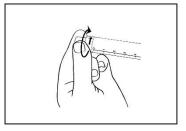
3) Twist off the end cap. Do not touch the exposed luer connection in order to avoid contamination.
